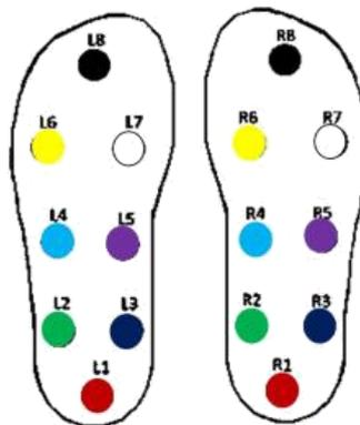
Figure 2: Placement of different sensors under feet.
