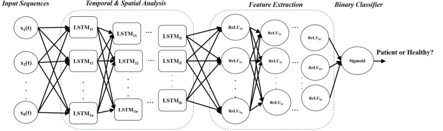
Figure 4: The proposed architecture for classifying patients and healthy persons by investigating the gait cycle based on temporal and spatial analysis of different sensors sequences.
