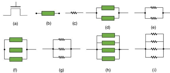
**Figure 6:** The steps of constructing a single nMOS transistor equivalent to the minimal Hammock network; (a)  $n$ -type single transistor, (b) minimal Hammock network  $H_{1,1}$ , (c) equivalent resistance circuit, (d) Hammock network  $H_{2,1}$ , (e) equivalent resistance circuit with redundancy of 2, (f) Hammock network  $H_{3,1}$ , (g) equivalent resistance circuit with redundancy of 3, (h) Hammock network  $H_{4,1}$ , (i) equivalent resistance circuit with redundancy of 4
