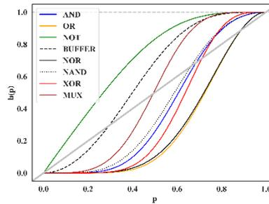
Figure 16: Reliability plots of basic logical gates along with 2:1 multiplexer according to the probability of failure in the switching function of transistors ( $p$ )
