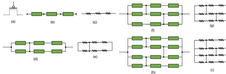
**Figure 7:** The steps of constructing a single pMOS transistor with the help of the minimal Hammock equivalent network; (a)  $p$ -type single transistor, (b) minimal Hammock network  $H_{1,3}$ , (c) equivalent resistance circuit, (d) Hammock network  $H_{2,3}$ , (e) equivalent resistance circuit with redundancy of 2, (f) Hammock network  $H_{3,3}$ , (g) circuit resistance equivalent to redundancy of 3, (h) Hammock network  $H_{4,3}$ , (i) resistance circuit equivalent to redundancy of 4
