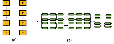
**Figure 12:** (a) Block diagram of XOR gate; (b) minimal Hammock network of XOR gate with redundancy of 2
