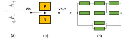
**Figure 8:** (a) Transistor arrangement of inverter gate; (b) Block diagram of the inverter; (c) Minimal Hammock network of the inverter with redundancy of 2
