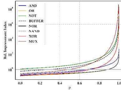
**Figure 18:** Reliability improvement index (RII) for basic logical gates along with 2:1 multiplexer according to the probability of failure in the switching function of transistors ( $p$ ); the vertical axis is assumed to be logarithmic.
