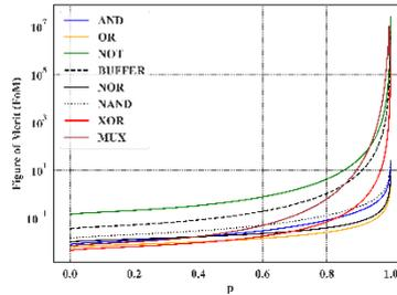
**Figure 19:** The figure of merit (FoM) index for basic logical gates along with a 2:1 multiplexer according to the probability of failure in the switching performance of transistors ( $p$ ); the vertical axis is logarithmic.
