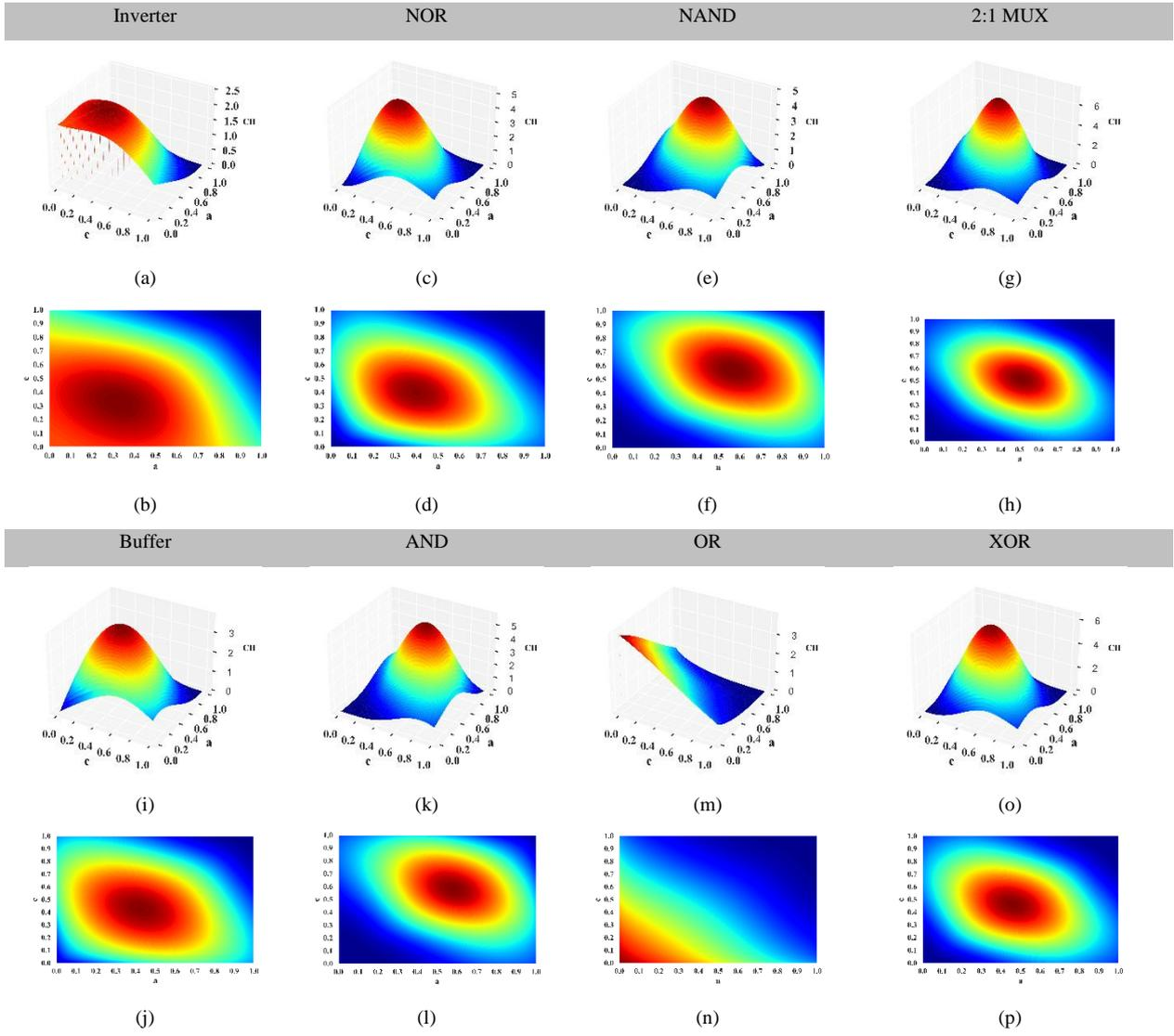
**Figure 23:** The channel capacity improvement index (CII) for basic logical gates along with 2:1 multiplexer; The values shown are normalized to the non-redundant Hammock channel capacity index,  $H_{1,1}$ ; For each circuit, the corresponding contour diagram is drawn for the sake of greater clarity.
