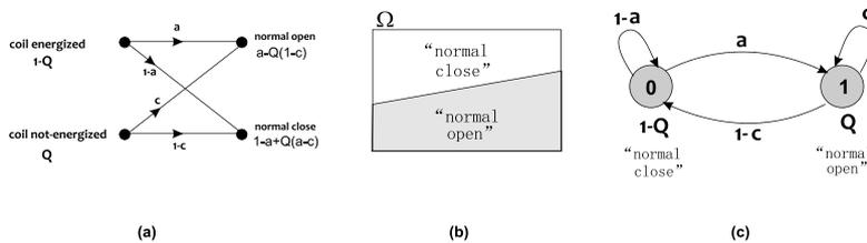
Figure 3: (a) illustration of a binary channel corresponding to a switching element (relay/transistor);  $Q$  is the probability of the coil being in an energized state and  $1-Q$  is the probability of its complement; (b) the Bayesian probability space corresponding to the normal-open (NO) and normal-close (NC) states; (c) state transition diagram corresponding to the binary channel depicted in (a)
